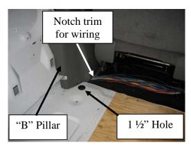
For neatness of wiring, route all cables down driver-side "B" pillar. If going under hood for power to console, drill hole at location above.
